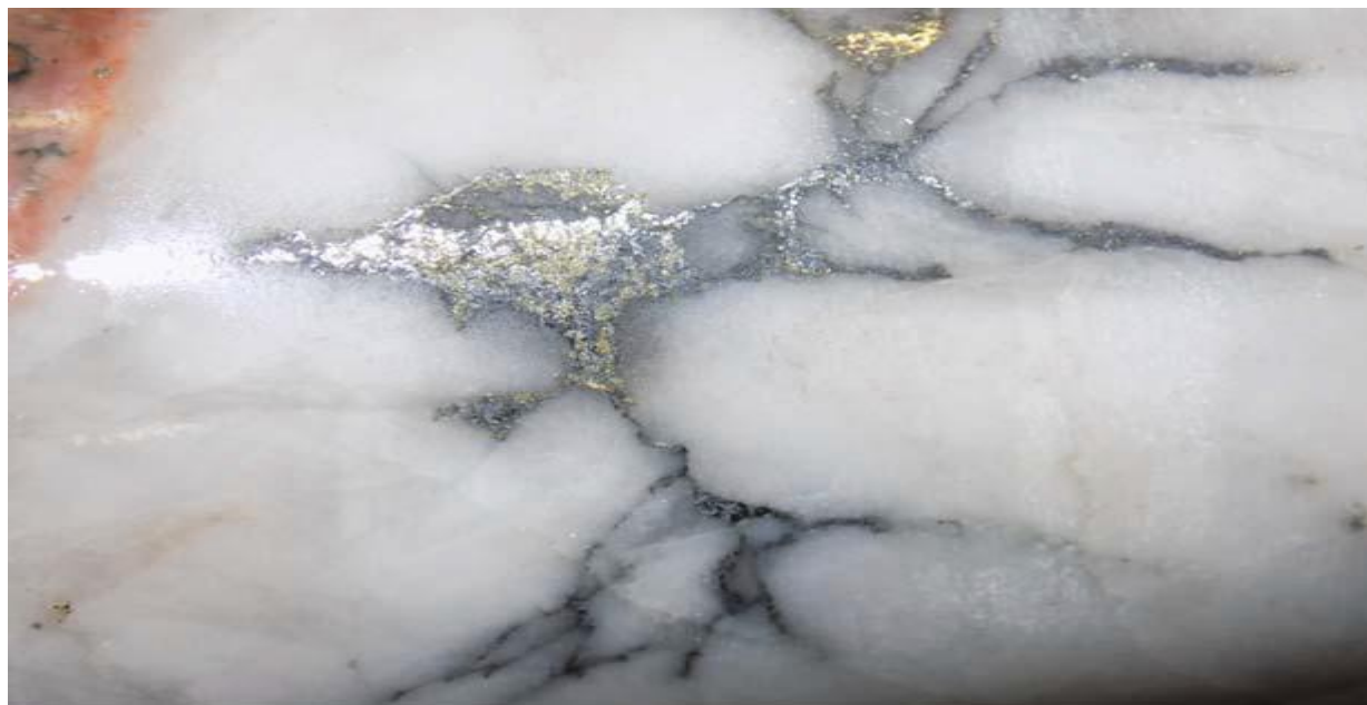
Figure 7-3 Au-Bi-Te stringers in quartz vein from 54.6 m, MG-14-12.
