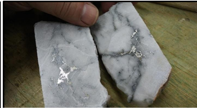
Gold Telluride Stringers @ 69.7m in Split Core
