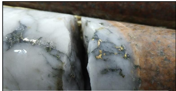
Visible Gold and Gold Tellurides @ 69.7m
